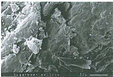
Pic 1: Scanning Electron Microscope of Surface of Sugar Beet Pellet.
